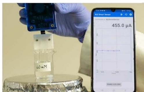
Fig. 1 Portable OECT sensor coupled to a portable electronic readout.
